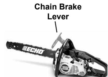
**⚠ WARNING!** It is the responsibility of the owner or operator to ensure that the brake is serviced, adjusted, and tested in accordance with the instructions as detailed in your instruction manual in order to ensure that the brake performance is maintained in compliance with ANSI B175.1- 2000, which stipulates that the brake shall stop the chain in a maximum of 0.15 seconds after activation (0.12 Average).
